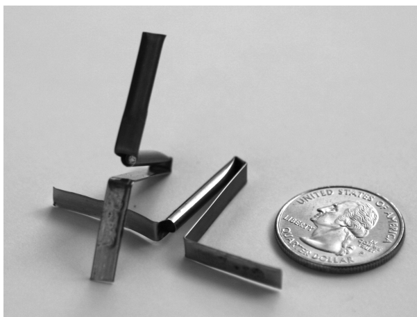
Figure 2.4: Two Alvatec alkali metal vapor sources with a United States quarter dollar coin for size comparison.
